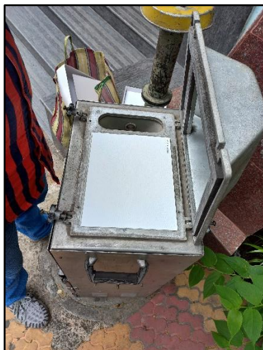
B. Placement of air filter in air monitoring machine
