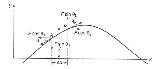
We have studied that the wave disturbance travels from one particle to another due to their masses (or inertia) and the factor responsible for the periodic motion of the particle is the elasticity of the medium. For a stretched string, the elasticity is measured by the tension F in it and the inertia is measured by mass per unit length or linear mass density,m.
