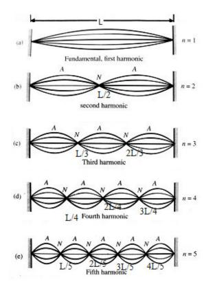
It means, in the nth mode, dx element of string vibrates simple harmonically
