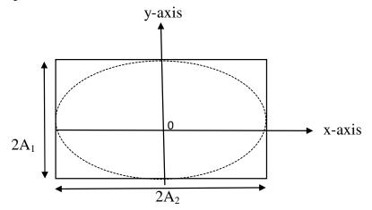
In case the amplitudes of the two individual SHMs are equal,  $A_1 = A_2 = A$ , i.e. the major and the minor axes are equal, then the ellipse reduces to acircle.
