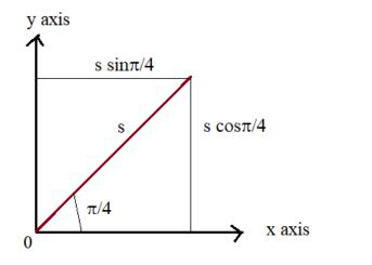
Components along X- axis :  $\frac{S}{\sqrt{2}} + A \sin\omega t = \frac{B\sin\omega t}{\sqrt{2}} + A \sin\omega t = \left(A + \frac{B}{\sqrt{2}}\right)\sin\omega t$ Component along Y-axis:  $\frac{S}{\sqrt{2}} = \frac{B\sin\omega t}{\sqrt{2}}$
