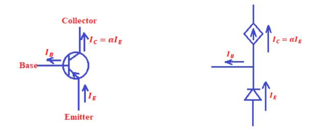
In active region Emitter-Base junction is forward biased i.e.  $V_{EB} > 0$  i.e.  $V_E - V_B > 0$ Collector-Base junction is reverse biased i.e.  $V_{CB} < 0$  i.e.  $V_C - V_B < 0$  Since the Base-Emitter junction is forward biased, the voltage is typically 0.6 to 0.75 V
