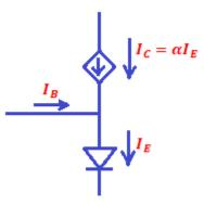
In active region Emitter-Base junction is forward biased i.e.  $V_{BE} > 0$  i.e.  $V_B - V_E > 0$ Collector-Base junction is reverse biased i.e.  $V_{BC} < 0$  i.e.  $V_B - V_C < 0$  Equivalent circuit of PNP transistor
