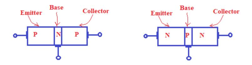
It consists of a silicon or germanium single crystal containing two pn junctions In beginning, junction transistors were manufactured by the two classical methods
