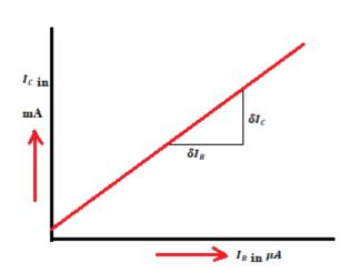
$$h_{fe} = \frac{\delta I_C}{\delta I_B}\Big|_{V_{CE}} = \beta_{ac}$$
