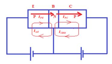
In PNP transistor collector-base junction is reverse biased for majority charged carriers but it is forward biased for thermally generated minority carriers.
