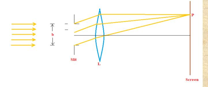
Where  $\theta$  is the angle at which the waves diffracted from the source. Corresponding phase difference
