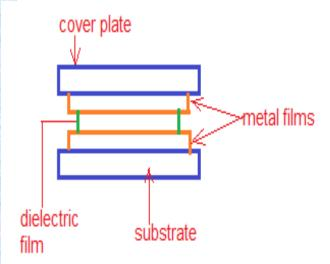
A thin metallic film, usually aluminium or silver is deposited on a substrate (glass). Then a thin layer of dielectric material such as cryolite (3NaF,AlF3) is deposited over this. This structure is This structure is again covered by another metallic film and another glass plate is placed over it. Thus a Fabry-Perot structure is formed between
