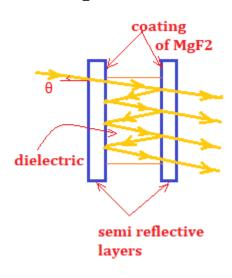
For chromatic light, transparent beam shall interfere constructively i.e. the path difference should be integral multiple of wavelength.
