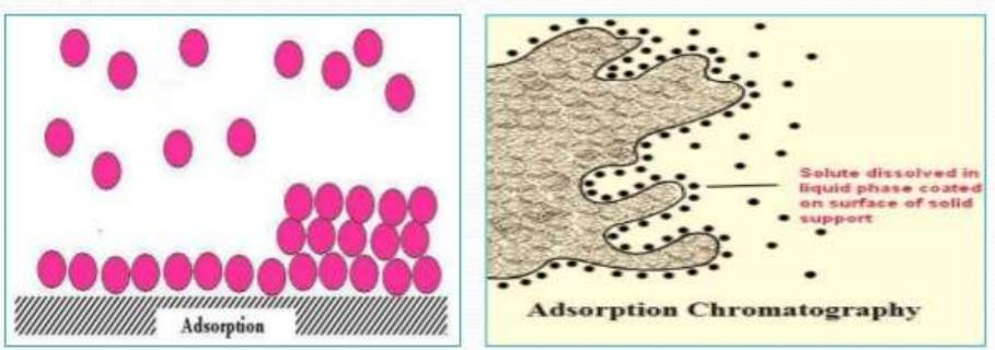
Principle of Adsorption Chromatography involves competition of components of sample mixture for active site on adsorbent. These active sites are formed in molecule due to
