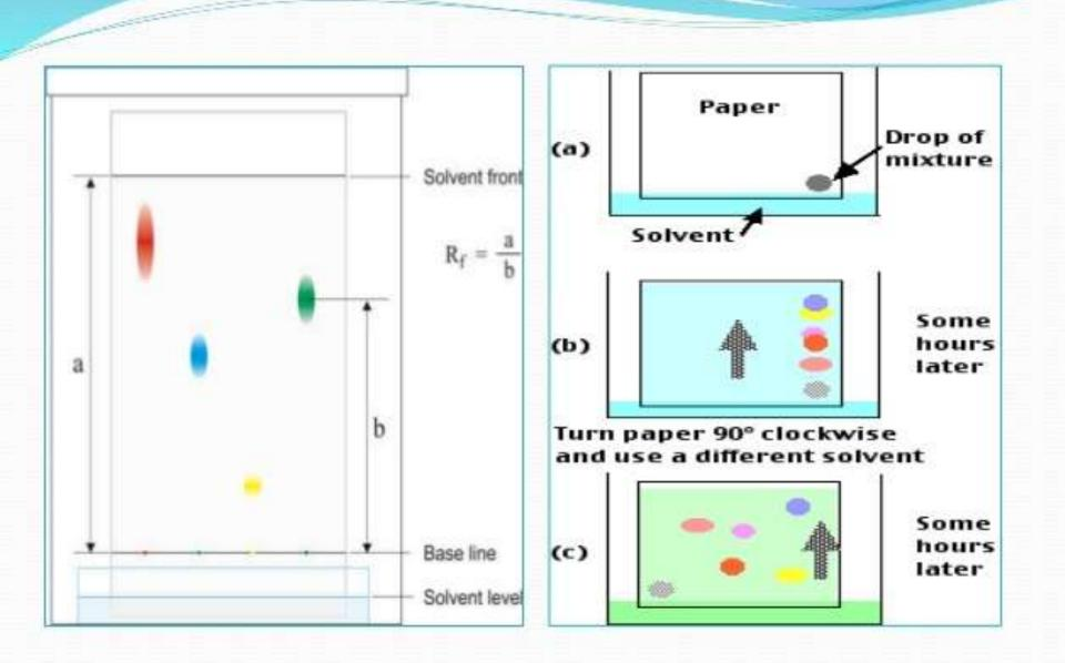
The principle involved is partition chromatography where in the substances are distributed or partitioned between to liquid phases. One phase is the water which is held in pores of filter paper used and other phase is that of mobile phase which moves over the paper. The compounds in the mixture get separated due to differences in their affinity towards water(in stationary phase) and mobile phase solvents during the movement of mobile phase under the capillary action of pores in the paper.
