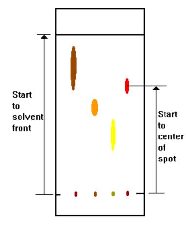
The Rf (retention factor) value for each spot should be calculated. It is characteristic for any given compound on the same stationary phase using the same mobile phase for development of the plates.
