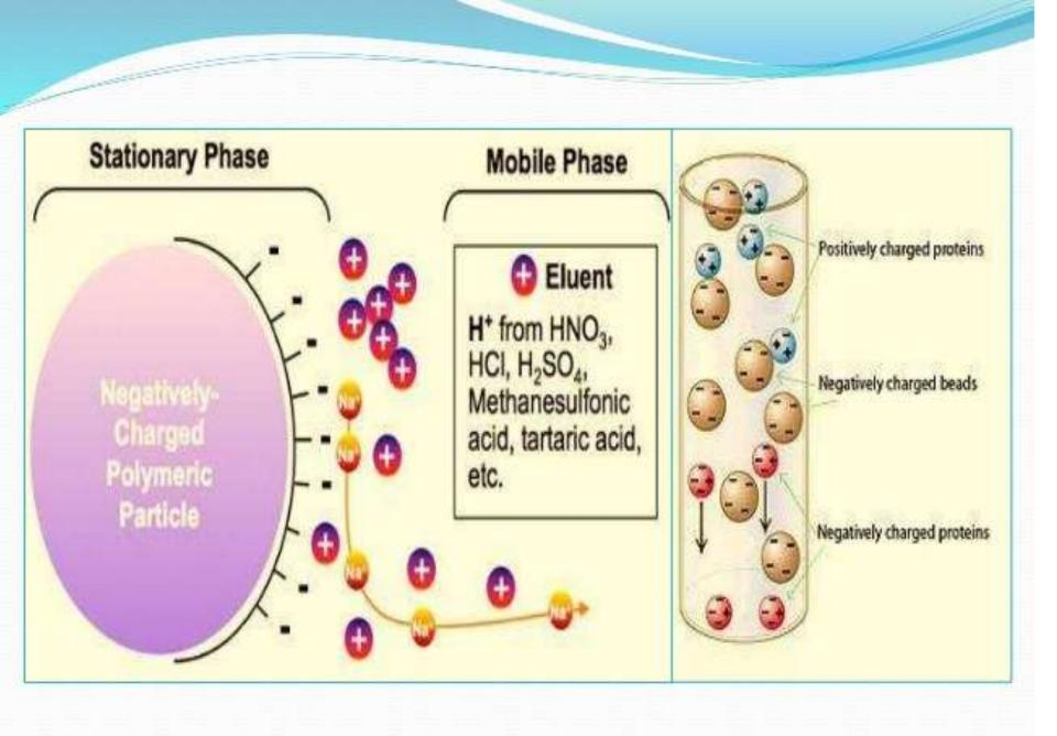
Ion Exchange Chromatography is based on the relative retention of the ions during their progress through an ion exchange column which has functional group of opposite charge attached to its surface. The stronger the charge on the ion, the greater is the retention time in the column.
