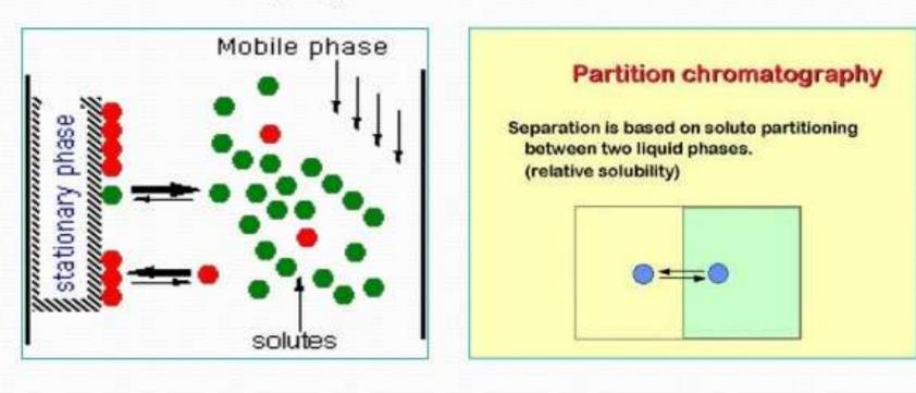
Separation of components of a sample mixture occurs because of partition. Stationary phase is coated with a liquid which is immiscible in mobile phase.
