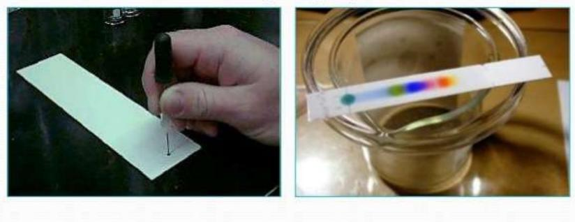
Similar to other chromatographic methods TLC is also based on the principle of separation. The separation depends on the relative affinity of compounds towards stationary and mobile phase. The compounds under the influence of mobile phase (driven by capillary action) travel over the surface of stationary phase. During this movement the compounds with higher affinity to stationary phase travel slowly while the others travel faster. Thus separation of components in the mixture is achieved.
