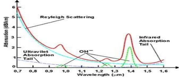
According to Rayleigh scattering loss is inversely proportional to the fourth power of the wavelength i.e.,  $1 / \lambda^4$ .
