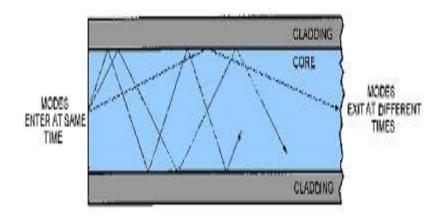
The total time delay between the higher order mode (mode that travel's longest path) and zero order mode (mode that shortest longest path),
