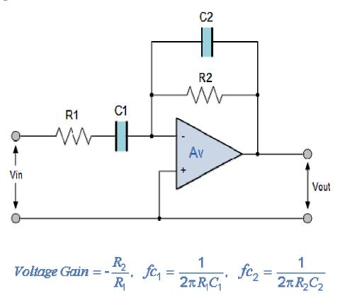
This type of band pass filter is designed to have a much narrower pass band. The centre frequency and bandwidth of the filter is related to the values of R1, R2, C1 and C2. The output of the filter is again taken from the output of the op-amp.
