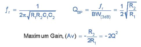
We can see then that the relationship between resistors,  $R_1$  and  $R_2$  determines the band pass "Q-factor" and the frequency at which the maximum amplitude occurs, the gain of the circuit will be equal to  $-2Q^2$ . Then as the gain increases so to does the selectivity. In other words, high gain – high selectivity.
