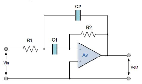
This active band pass filter circuit uses the full gain of the operational amplifier, with multiple negative feedback applied via resistor,  $R_2$  and capacitor  $C_2$ . Then we can define the characteristics of the IGMF filter as follows:
