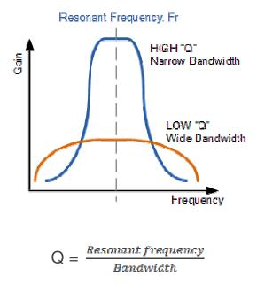
Then for our simple example above the quality factor "Q" of the band pass filter is given as:
