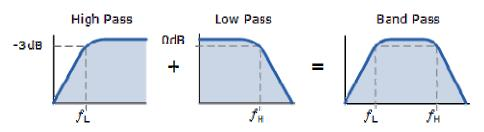
The higher corner point  $(f_{\rm H})$  as well as the lower corner frequency cut-off point  $(f_{\rm L})$  are calculated the same as before in the standard first-order low and high pass filter circuits. Obviously, a reasonable separation is required between the two cut-off points to prevent any interaction between the low pass and high pass stages. The amplifier also provides isolation between the two stages and defines the overall voltage gain of the circuit.
