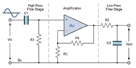
This cascading together of the individual low and high pass passive filters produces a low "Q-factor" type filter circuit which has a wide pass band. The first stage of the filter will be the high pass stage that uses the capacitor to block any DC biasing from the source. This design has the advantage of producing a relatively flat asymmetrical pass band frequency response with one half representing the low pass response and the other half representing high pass response as shown.
